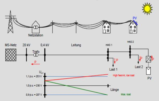
Voltage Problems were previously associated with costly grid development involving increased amounts of copper, new cables and more powerful transformers.
